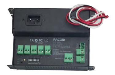
The PACOM 8308 Intelligent Uninterruptible Power Supply (UPS) provides a regulated 10.5 to 17.5VDC supply for powering controllers, peripheral devices and charging backup batteries. It can be remotely configured, controlled and monitored by PACOM Security Managment Software. A PACOM Controller acts as an interface to the 8308 UPS via RS485.
